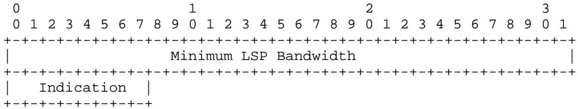
The Minimum LSP Bandwidth is encoded in a 4-octet field in the IEEE floating point format. The units are bytes (not bits!) per second. The indication whether the interface supports Standard or Arbitrary SONET/SDH is encoded as 1 octet. The value of this octet is 0 if the interface supports Standard SONET/SDH, and 1 if the interface supports Arbitrary SONET/SDH.
