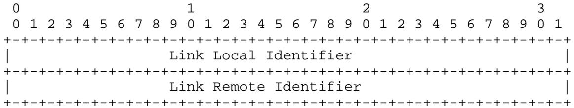
The Link Local/Remote Identifiers sub-TLV MUST NOT occur more than once within the extended IS reachability TLV. If the Link Local/Remote Identifiers sub-TLV occurs more than once within the extended IS reachability TLV, the receiver SHOULD ignore all these sub-TLVs.
