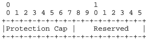
The first octet is a bit vector describing the protection capabilities of the link (see Section 2.2, "Link Protection Type", of [GMPLS-ROUTING]). They are:
