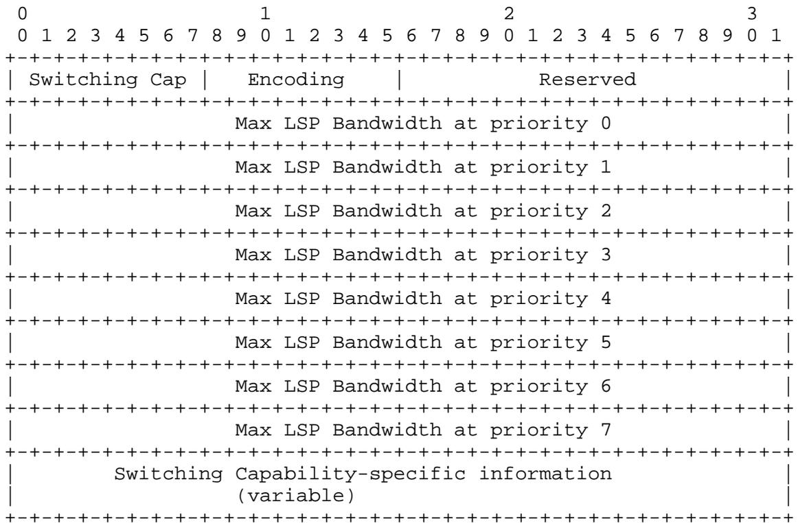
The Switching Capability (Switching Cap) field contains one of the following values:
