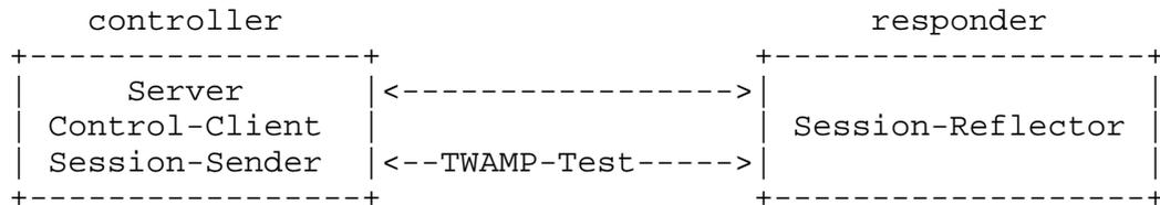
This example provides a simple architecture for responders where their role will be to simply act as light test points in the network. The controller establishes the test session with the Server through non-standard means. After the session is established, the controller transmits test packets to the responder. The responder follows the Session-Reflector behavior of TWAMP as described in section 4.2 with the following exceptions.
