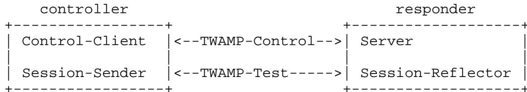
This example provides an architecture that supports the full TWAMP standard. The controller establishes the test session with the responder through the TWAMP-Control protocol. After the session is established, the controller transmits test packets to the responder. The responder follows the Session-Reflector behavior of TWAMP as described in Section 4.2.
