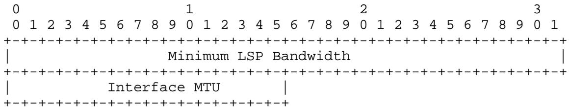
The Minimum LSP Bandwidth is encoded in a 4-octet field in the IEEE floating point format. The units are bytes (not bits!) per second. The Interface MTU is encoded as a 2-octet integer, and carries the MTU value in the units of bytes.
