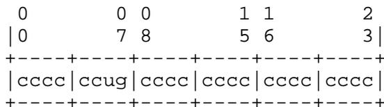
written in Internet standard bit-order , where "u" is the universal/local bit, "g" is the individual/group bit, and "c" are the bits of the company\_id. Appendix A: "Creating EUI-64 based Interface Identifiers" provides examples on the creation of different EUI-64 based interface identifiers.
