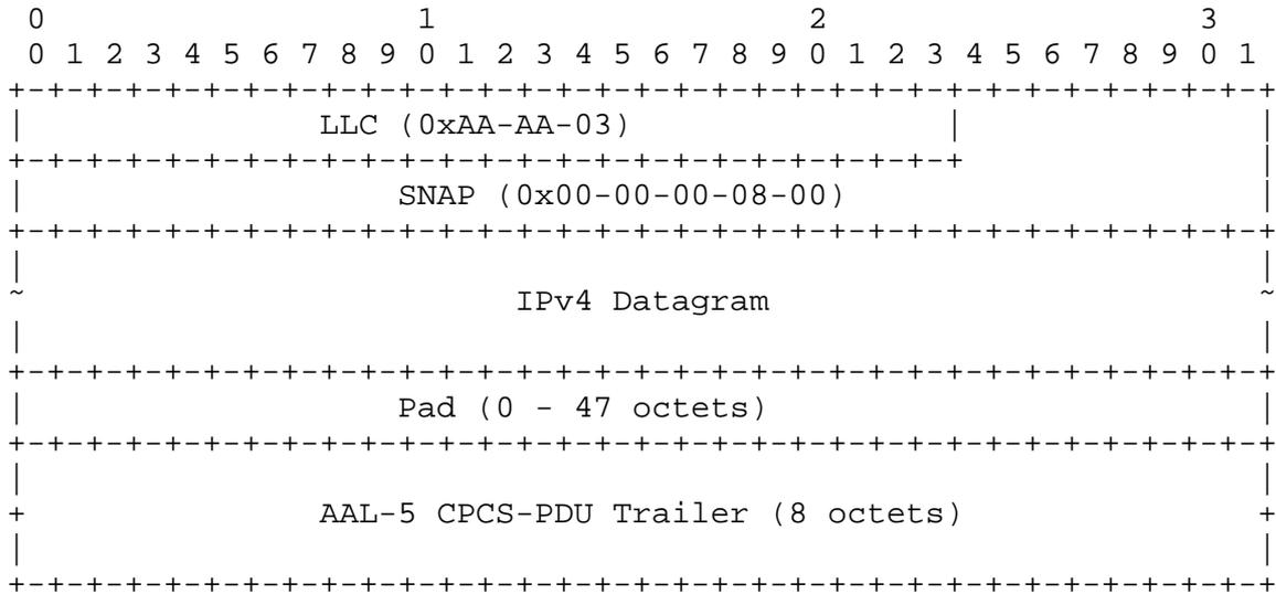
The maximum transmission unit (MTU) of an IPv4 datagram using the default encapsulation is 1500 octets.
