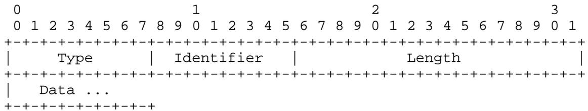
A summary of the Bandwidth Allocation Protocol datagram Response packet format is shown below. The fields are transmitted from left to right.
