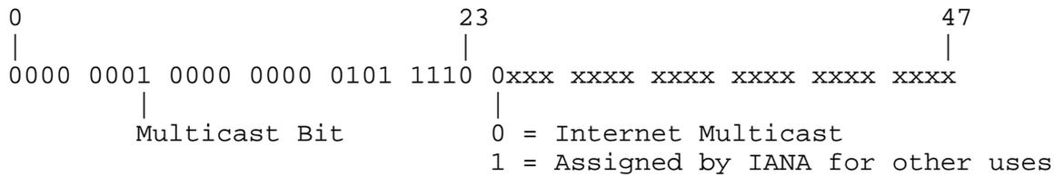
The latter representation corresponds to the Internet standard bit-order, and is the format that most programmers have to deal with. Using this representation, the range of Internet Multicast addresses is:
