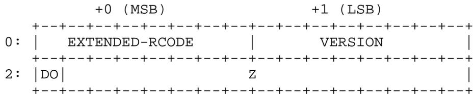
Setting the DO bit to one in a query indicates to the server that the resolver is able to accept DNSSEC security RRs. The DO bit cleared (set to zero) indicates the resolver is unprepared to handle DNSSEC security RRs and those RRs MUST NOT be returned in the response (unless DNSSEC security RRs are explicitly queried for). The DO bit of the query MUST be copied in the response.
