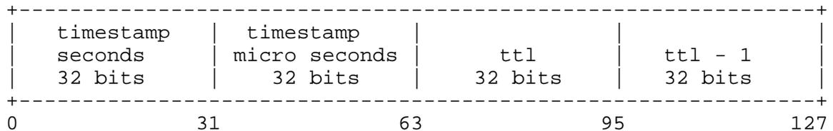
The fields are stored in XDR (external data representation) format. The timestamp encodes the time since midnight, January 1, 1970. These 128 bits of data are then encrypted in the DES CBC mode, using the conversation key for the session, and with an initialization vector of 0. This yields:
