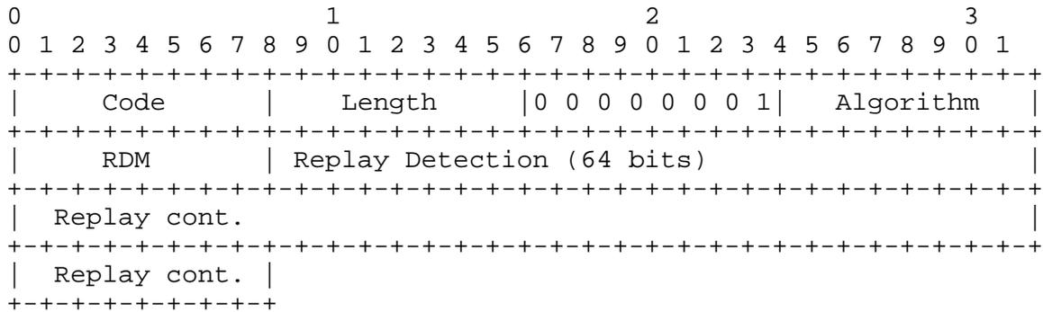
The format of the authentication information in a DHCPOFFER, DHCPREQUEST or DHCPACK message for delayed authentication is:
