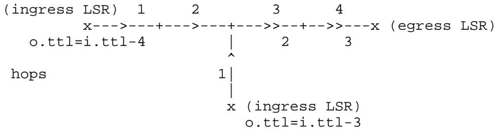
Frame Relay Multicast -- TTL calculated at egress
