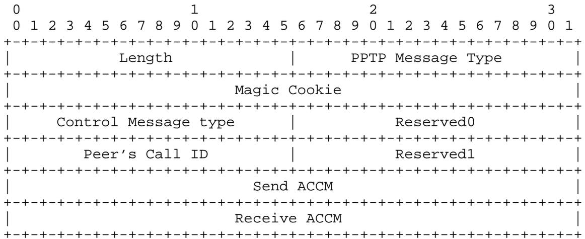
Length                              Total length in octets of this PPTP message, including the entire PPTP header.
