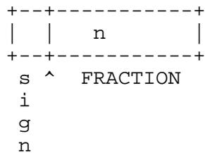
Where the sign occupies the most significant bit of the coordinate followed by bits of numerical information (initial implementation of NGP requires N=15). Negative numbers are represented by 2's complement. Conversion to device coordinates is accomplished by:
