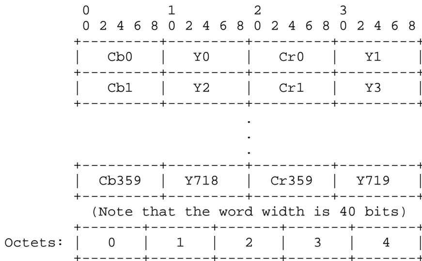
The octets shown in these diagrams are transmitted in network byte order, that is, left-to-right as shown.
