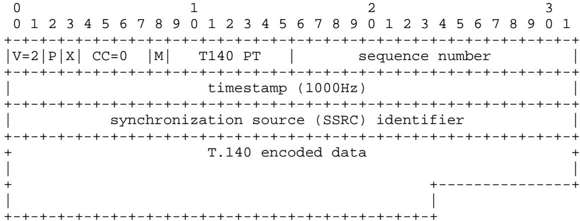
This is an example of an RTP packet with one redundant T140block.
