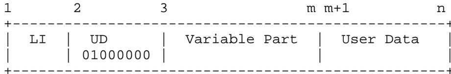
LI (octet 1) - the length of the header including parameters, but excluding the LI and user data, with a maximum value of 254
