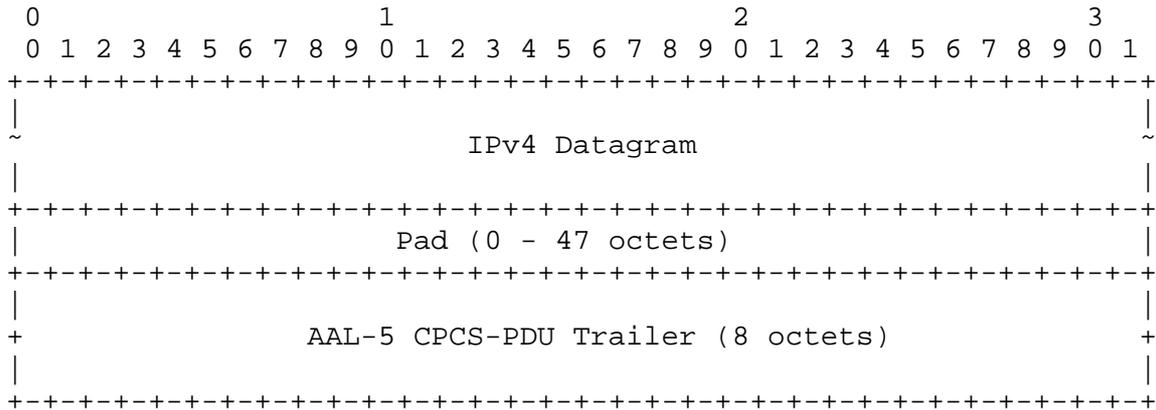
The MTU of an IPv4 datagram using Flow Type 0 encapsulation is 1500 octets.
