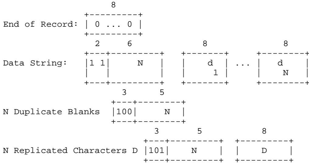
HASP is concerned only with 8-bit bytes. However, there is a provision (which was never implemented) in the Multileaving Protocol to set the unit of the counts N as 1 byte, 2 bytes, or 4 bytes.
