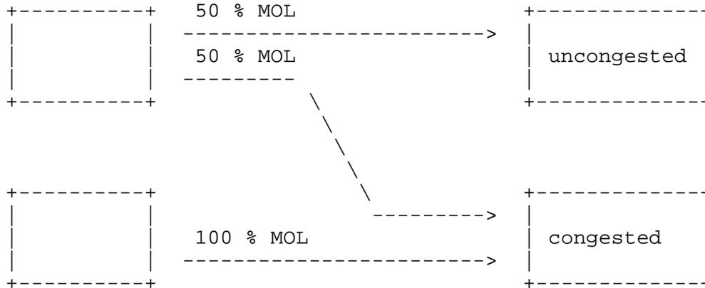
Both source transmitters MUST transmit the exact number of test frames. The first source MUST transmit test frames at the MOL with the destination address of the two receive ports in an alternating order. The first test frame to the uncongested receive port, second test frame to the congested receive port, then repeat. The second source transmitter MUST transmit test frames at the MOL only to the congested receive port.
