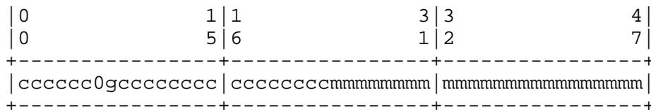
where "c" are the bits of the assigned company\_id, "0" is the value of the universal/local bit to indicate global scope, "g" is individual/group bit, and "m" are the bits of the manufacturer-selected extension identifier. The interface identifier would be of the form:
