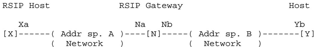
Hosts X and Y belong to different addressing realms A and B, respectively, and N is an RSIP gateway (which may also perform NAT functions). N has two interfaces: Na on address space A, and Nb on address space B. N may have a pool of addresses in address space B which it can assign to or lend to X and other hosts in address space A. These addresses are not shown above, but they can be denoted as Nb1, Nb2, Nb3 and so on.
