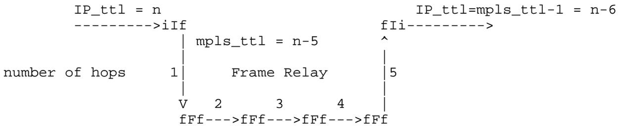
"iIf" is "ingress LSR" in Frame Relay LSP and calculates:  $mpls\_ttl = IP\_TTL - \text{number of hops} = n-5$
