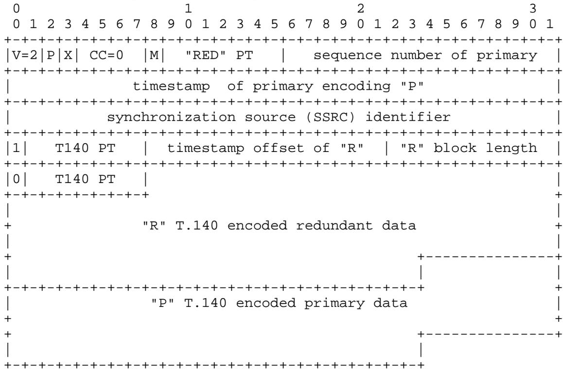
Figure: Examples of RTP text packets.
