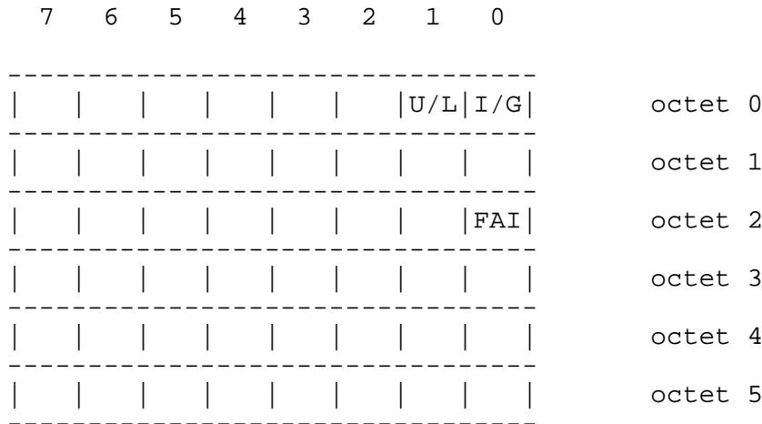
The low order bit of the high order octet is called the I/G bit. It signifies whether the address is an individual address (0) or a group address (1). This is comparable to the multicast bit in the DIX Ethernet addressing format.
