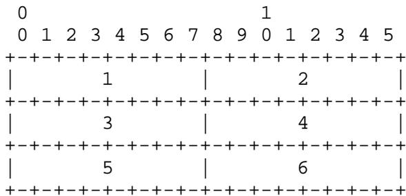
Whenever an octet represents a numeric quantity, the left most bit in the diagram is the high order or most significant bit. That is, the bit labeled 0 is the most significant bit. For example, the following diagram represents the value 170 (decimal).
