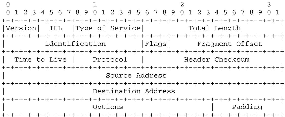
There are two ways to compress the IPv4 header
