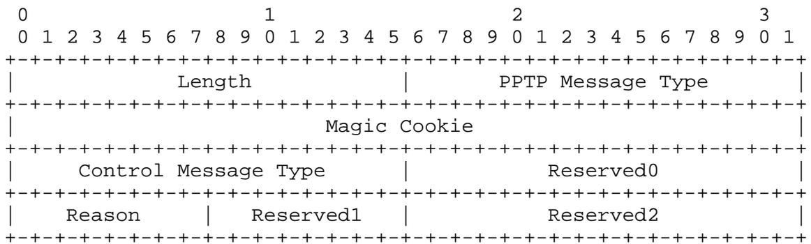
Length                      Total length in octets of this PPTP message, including the entire PPTP header.
