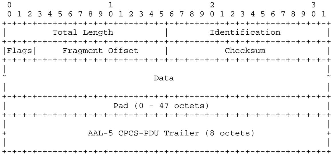
The MTU of the IPv4 datagram using Flow Type 1 encapsulation is 1484 octets (1500 octets minus the 16 octets specified above).
