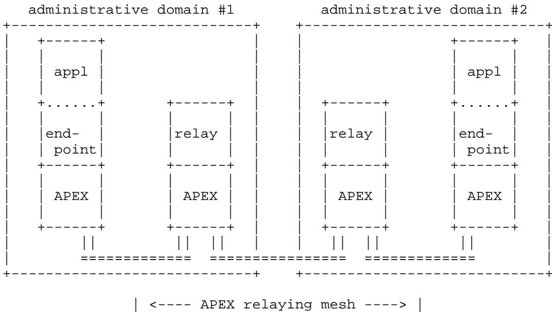
Note: relaying between administrative domains is configured using SRV RRs. Accordingly, the actual number of relays between two endpoints is not fixed.
