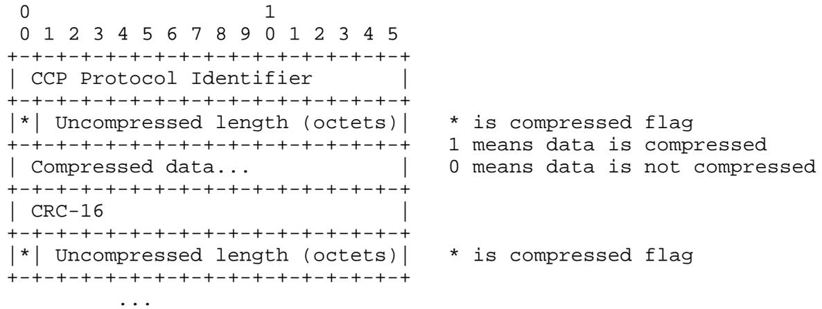
The CCP Protocol Identifier that starts the packet is always 0xfd. If PPP Protocol field compression has not be negotiated, it MUST be a 16-bit field.
