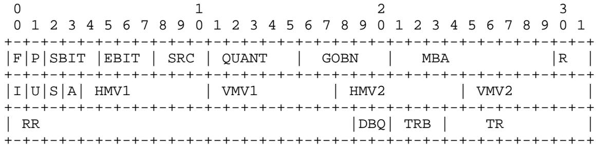
The following fields are defined the same as in mode B: F, P, SBIT, EBIT, SRC, QUANT, GOBN, MBA, R, I, U, S, A, HVM1, VMV1, HVM2, VMV2. The rest of the fields (TR, DBQ, TRB) are defined the same as in mode A, except field RR. The RR field takes 19 bits, and is currently reserved. It must be set to zero.
