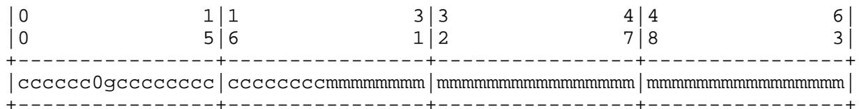
where "c" are the bits of the assigned company\_id, "0" is the value of the universal/local bit to indicate global scope, "g" is individual/group bit, and "m" are the bits of the manufacturer-selected extension identifier. The IPv6 interface identifier would be of the form:
