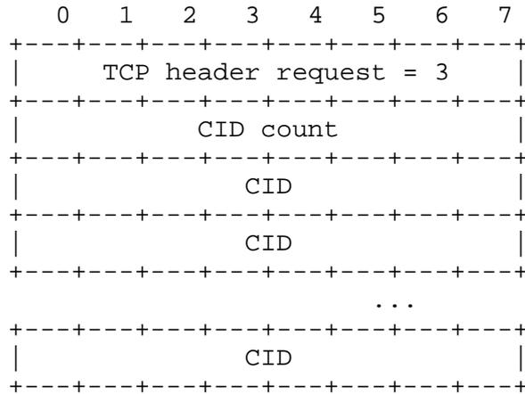
The first octet is a type code to allow the CONTEXT\_STATE packet type to be shared for other compression protocols that are (see [CRTP]) or may be defined in parallel with this one. When used for TCP header requests the type code has the value 3, and the remainder of the packet is a sequence of CIDs preceded by a one-octet count of the number of CIDs.
