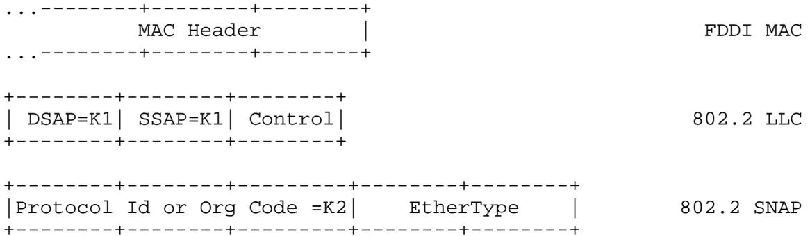
The total length of the LLC Header and the SNAP header is 8 octets.
