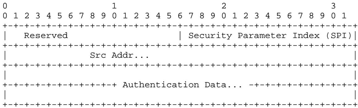
Security Parameter Index (SPI) can be thought of as an index into a table that maintains the keys and other information such as hash algorithm. Src and Dst communicate either offline using manual keying or online using a key management protocol to populate this table. The sending NHRP entity always allocates the SPI and the parameters associated with it.
