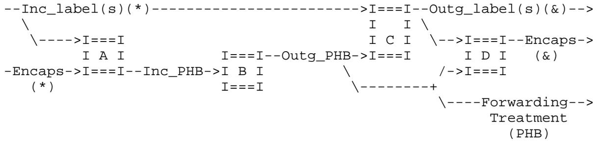
"Encaps" designates the Diff-Serv related information encoded in the MPLS Encapsulation layer (e.g., EXP field, ATM CLP, Frame Relay DE, 802.1 User\_Priority)
