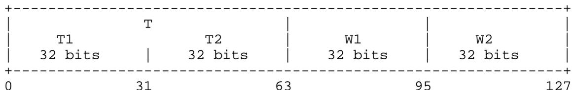
where T1, T2, W1, and W2 are all 32-bit quantities, and have some correspondence to the original quantities occupying their positions, but are now interdependent on each other for proper decryption. The 64 bit sequence comprising T1 and T2 is denoted by T.
