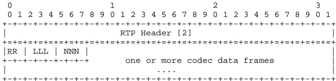
The RTP header has the expected values as described in [2]. The extension bit is not set and this payload type never sets the marker bit. The codec data frames are aligned on octet boundaries. When interleaving is in use and/or multiple codec data frames are present in a single RTP packet, the timestamp is, as always, that of the oldest data represented in the RTP packet. The other fields have the following meaning:
