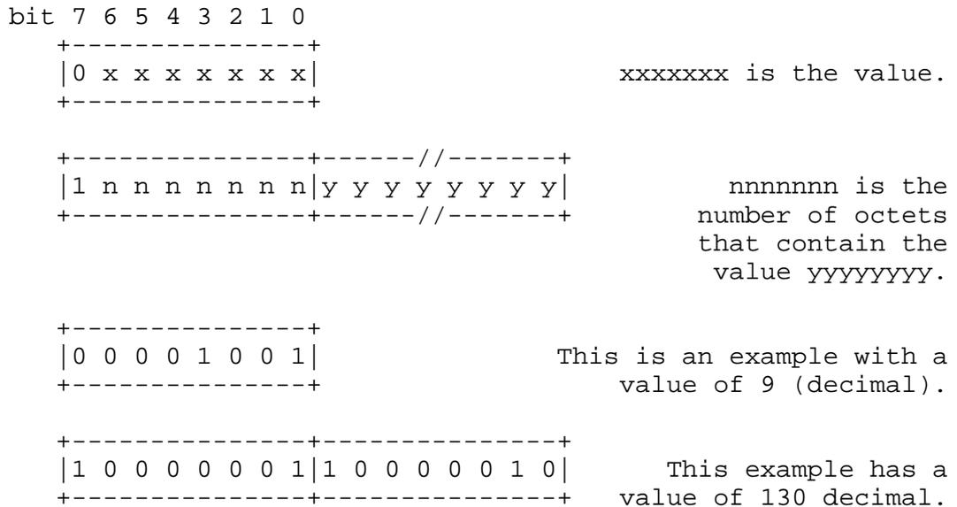
FIG. 5. ENCODING MECHANISM FOR QUALIFIERS AND LENGTH CODES
