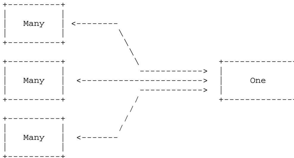
For every address, the testing device MUST send learning frames to allow the DUT/SUT to update its address tables properly.
