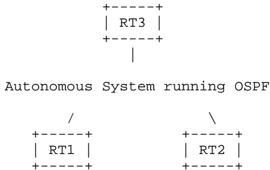
Both RT1 and RT2 have routes to an external network X and import it into the OSPF routing domain. RT3 is advertising the route to network X to other external BGP speakers. RT3
