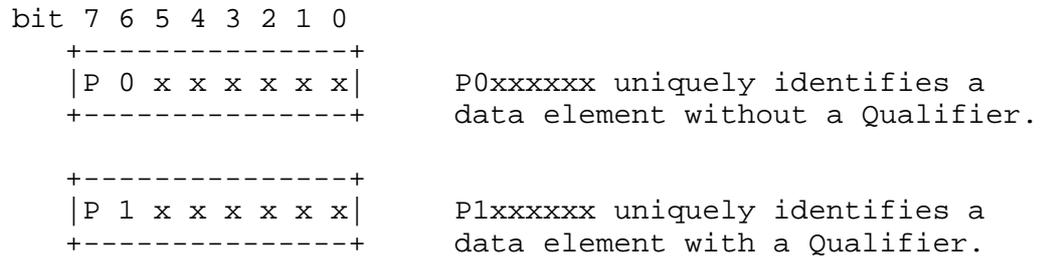
FIG. 4. STRUCTURE OF IDENTIFIER OCTETS
