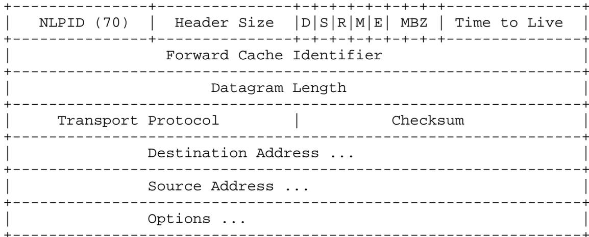
**NLPID:** The first byte (the network layer protocol identifier in OSI) is an 8 bit constant 70 (hex). This corresponds to Internet Version 7.
