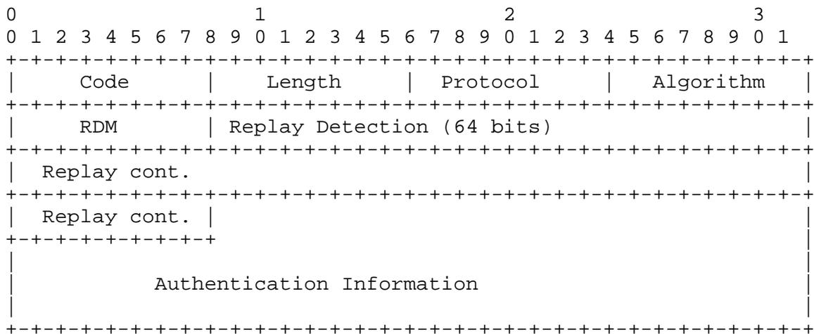
The code for the authentication option is 90, and the length field contains the length of the protocol, RDM, algorithm, Replay Detection fields and authentication information fields in octets.
