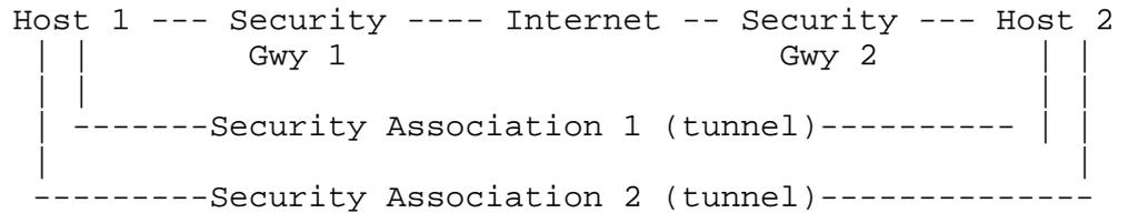
2. one endpoint of the SAs is the same -- The inner and outer tunnels could each be either AH or ESP.
