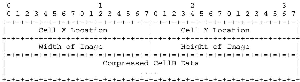
All fields are 16-bit unsigned integers in network byte order, and are placed at the beginning of the payload for each RTP packet. The Cell X and the Cell Y Location coordinates are expressed as cell coordinates, not pixel coordinates. Since cells represent 4x4 blocks of pixels, the X or Y dimension of the cell coordinates range in value from 0 through 1/4 of the of the same dimension in pixel coordinates.
