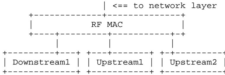
As can be seen from this example, the RF MAC interface is layered on top of the downstream and upstream interfaces.
