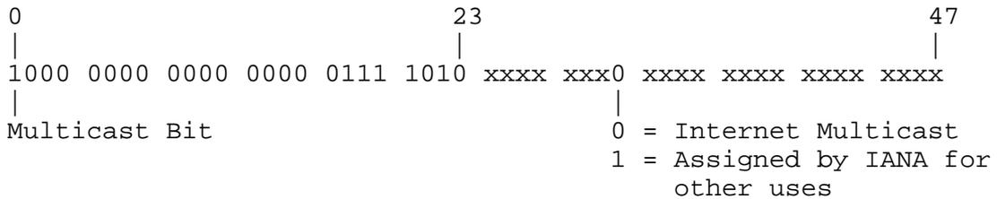
Appearance in memory (bits transmitted right-to-left within octets, octets transmitted left-to-right):
