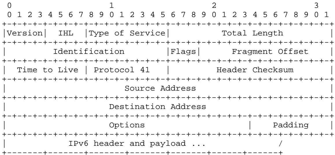
If there are IPv4 options, then padding SHOULD be added to the IPv4 header such that the IPv6 header starts on a boundary that is a 32-bit offset from the end of the datalink header.
