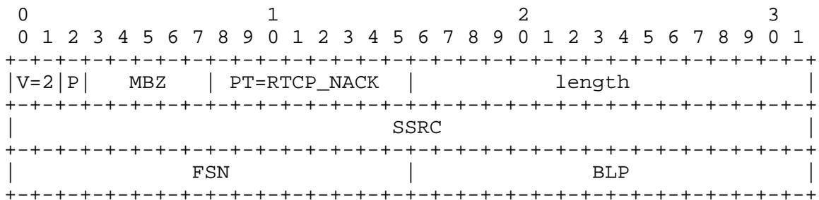
The various fields T, P, PT, length and SSRC are defined in the RTP specification [1]. The value of the packet type (PT) identifier is the constant RTCP\_NACK (193). SSRC is the synchronization source identifier for the sender of this packet.
