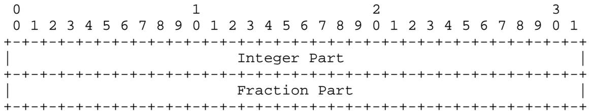
This format allows convenient multiple-precision arithmetic and conversion to Time Protocol representation (seconds), but does complicate the conversion to ICMP Timestamp message representation (milliseconds). The low-order fraction bit increments at about 0.2-nanosecond intervals, so a free-running one-millisecond clock will be in error only a small fraction of one part per million, or less than a second per year.
