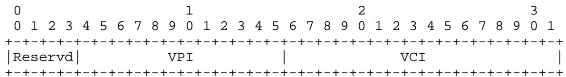
The low order 16 bits of the label correspond to the VCI, with the least significant bit of the Label field corresponding to the least significant bit of the VCI. If the link cannot support a full 16 bit VCI the unused bits of the VCI must be the most significant bits and they must be set to zero.
