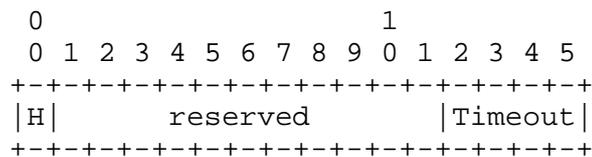
The Modem On-Hold Status AVP is a 16-bit quantity, containing two fields that indicate whether the client modem has placed the call on-hold and the maximum amount of time that the call is allowed to remain on-hold.
