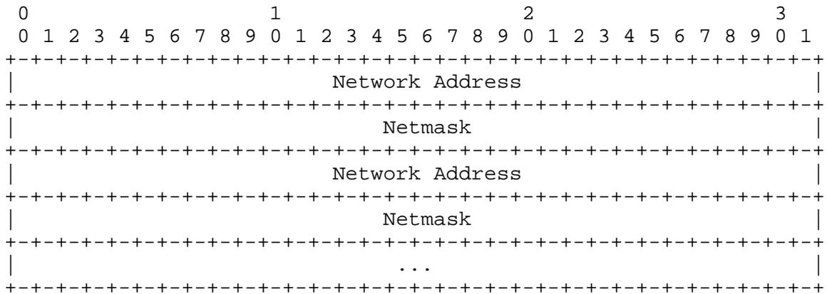
This is sent as the data part of the general packet format with the "Message Type" set to HNA\_MESSAGE, the TTL field set to 255 and Vtime set accordingly to the value of HNA\_HOLD\_TIME, as specified in section 18.3.
