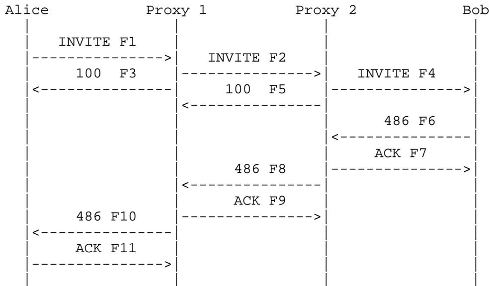
In this scenario, Bob is busy and sends a 486 Busy Here response to Alice's INVITE. Note that the non-2xx response is acknowledged on a hop-by-hop basis instead of end-to-end. Also note that many SIP UAs will not return a 486 response, as they have multiple line and other features.
