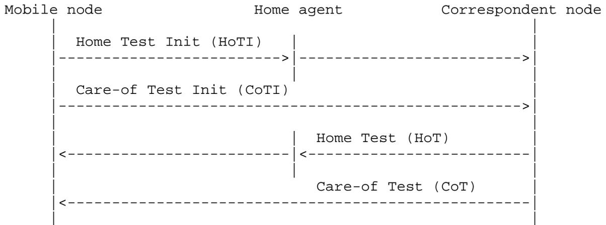
The Home and Care-of Test Init messages are sent at the same time. The procedure requires very little processing at the correspondent node, and the Home and Care-of Test messages can be returned quickly, perhaps nearly simultaneously. These four messages form the return routability procedure.
