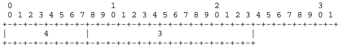
The length of the message is 3 octets which encompasses the one octet Type field and the two octet Length field.
