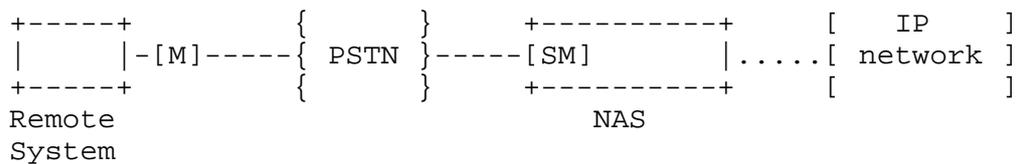
M is the client modem and may be an integral part of the Remote System. If this modem implements V.92, it can ask the server modem SM (a part of the NAS) whether the call can be placed on-hold for some period of time.
