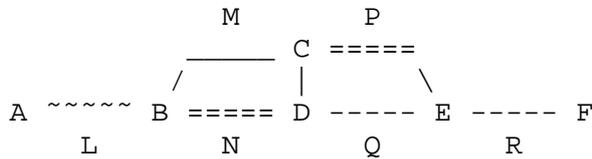
Say that the link MTU for link L is 9216; for links M, Q, and R, 4470; and for N and P, is 1500.
