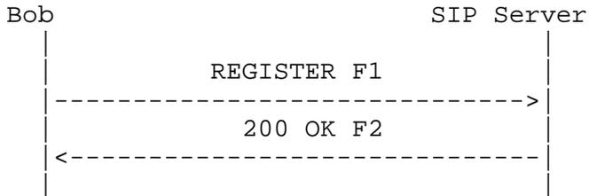
Bob sends a register request to the Proxy Server containing no Contact headers, indicating the user wishes to query the server for the user's current contact list. Since the user already has authenticated with the server, the user supplies authentication credentials with the request and is not challenged by the server. The SIP server validates the user's credentials. The server returns a response (200 OK) which includes the user's current registration list in Contact headers.
