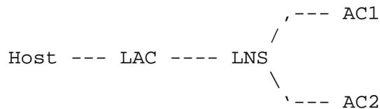
In this example, AC1 and AC2 are PPPoE access concentrators on a broadcast domain. Sequence of operation is as follows.
