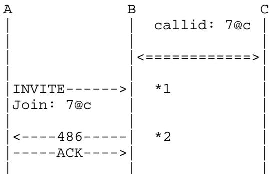
In this example B is Busy (does not want to be disturbed), and therefore does not wish to add A. B could also decline the request with a 603 response.
