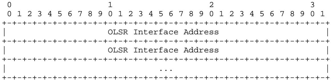
This is sent as the data-portion of the general packet format described in section 3.4, with the "Message Type" set to MID\_MESSAGE. The time to live SHOULD be set to 255 (maximum value) to diffuse the message into the entire network and Vtime set accordingly to the value of MID\_HOLD\_TIME, as specified in section 18.3.
