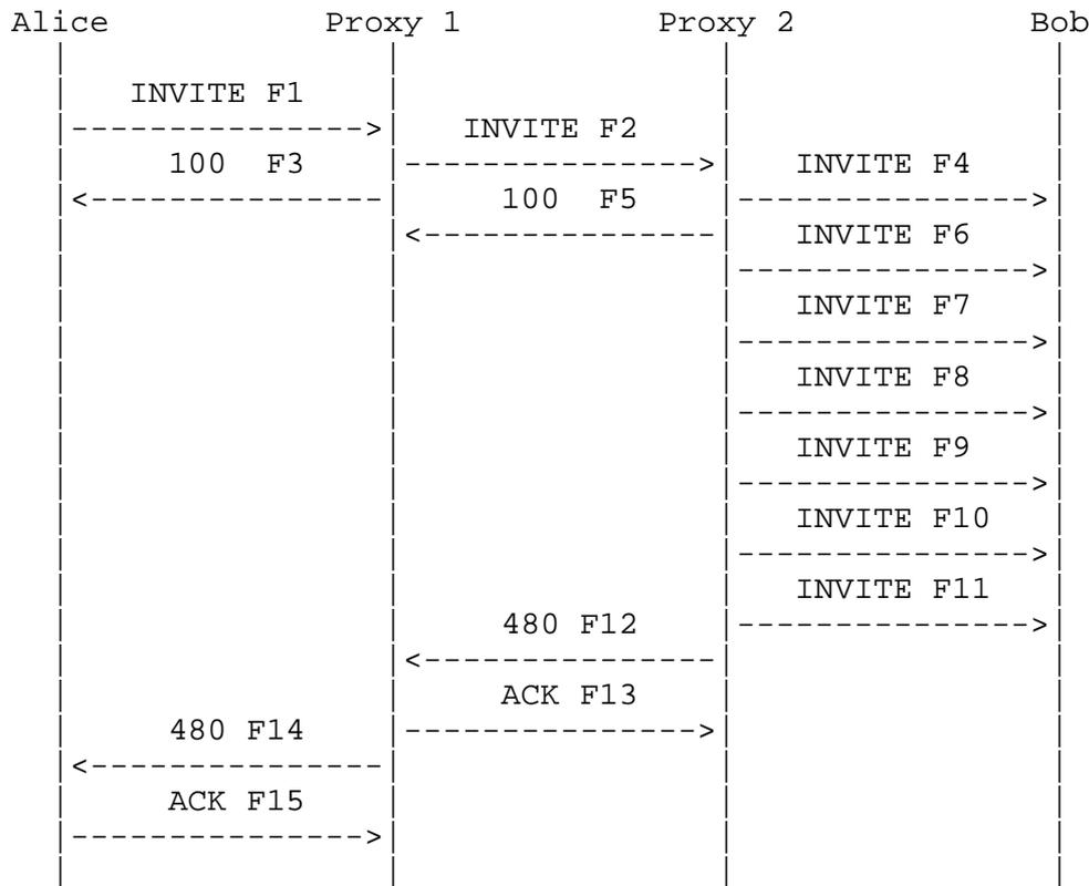
In this example, there is no response from Bob to Alice's INVITE messages being re-transmitted by Proxy 2. After the sixth re-transmission, Proxy 2 gives up and sends a 480 No Response to Alice.
