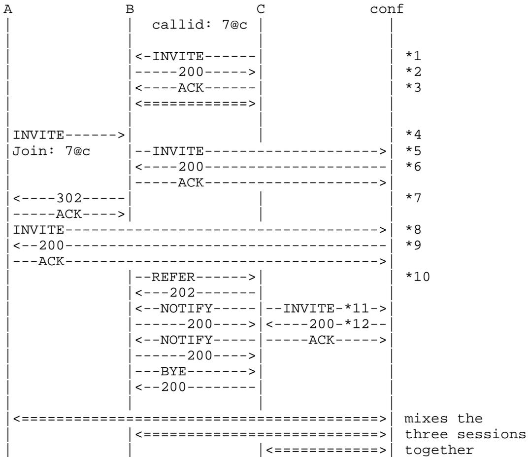
The conversation now appears identical to the locally mixed one from the example in the Introduction. Details of how the Join are implemented are transparent to A. B could have used 3rd party call control instead to move the necessary sessions.
