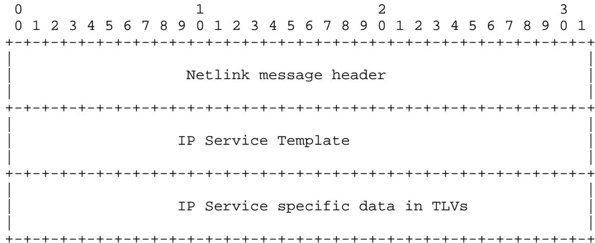
The Netlink message is used to communicate between the FEC and CPC for parameterization of the FECs, asynchronous event notification of FEC events to the CPCs, and statistics querying/gathering (typically by a CPC).
