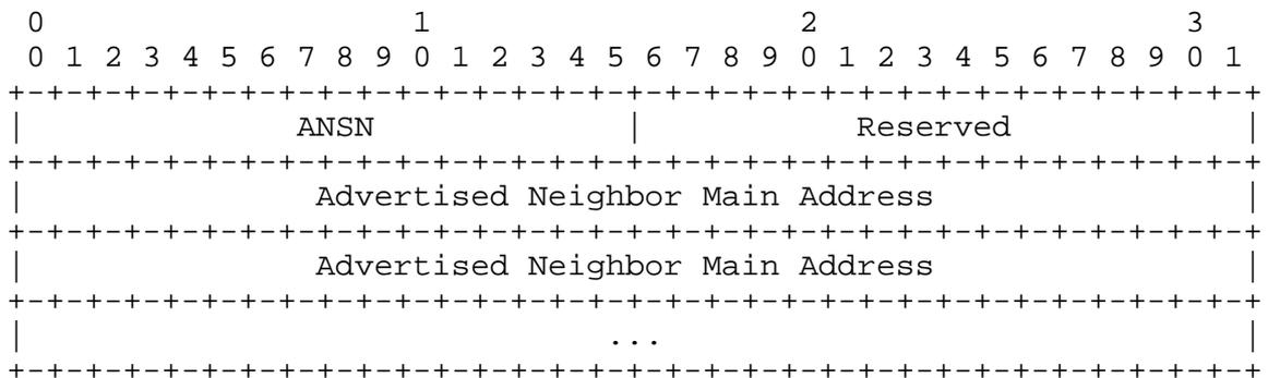
This is sent as the data-portion of the general message format with the "Message Type" set to TC\_MESSAGE. The time to live SHOULD be set to 255 (maximum value) to diffuse the message into the entire network and Vtime set accordingly to the value of TOP\_HOLD\_TIME, as specified in section 18.3.
