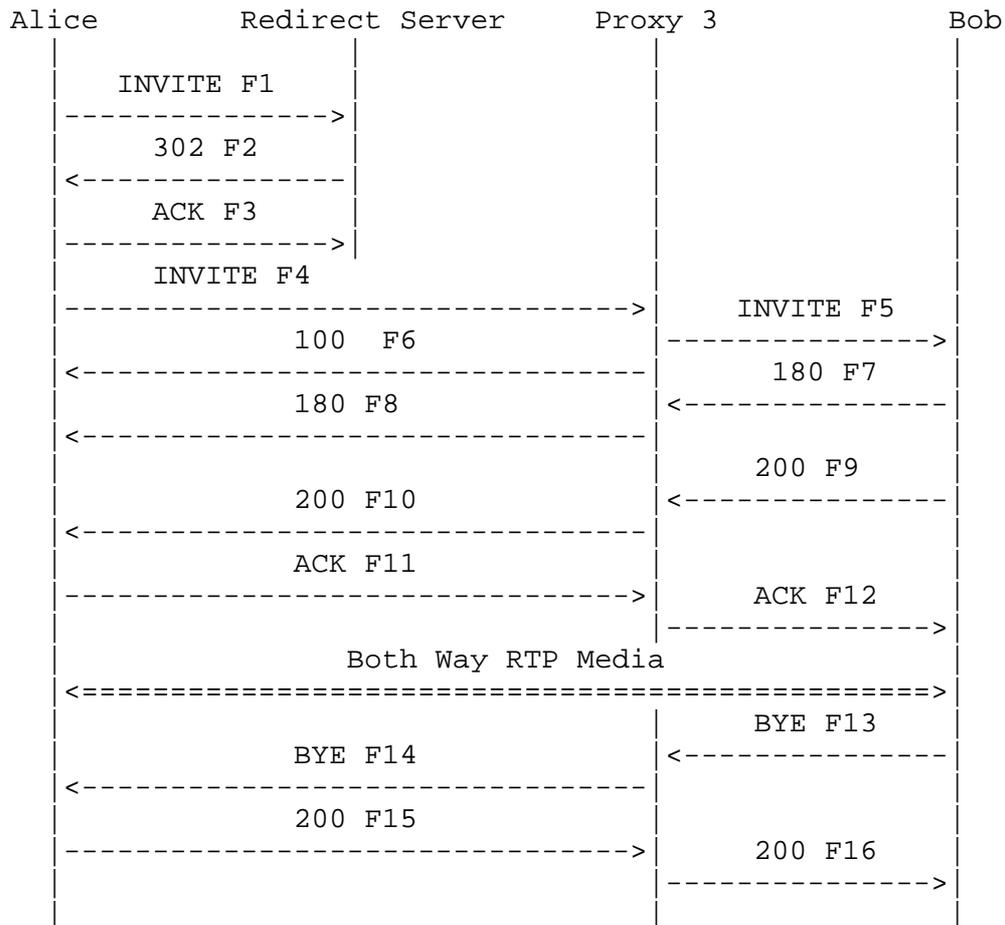
In this scenario, Alice places a call to Bob using first a Redirect server then a Proxy Server. The INVITE message is first sent to the Redirect Server. The Server returns a 302 Moved Temporarily response (F2) containing a Contact header with Bob's current SIP address. Alice then generates a new INVITE and sends to Bob via the Proxy Server and the call proceeds normally. In this example, no SDP is present in the INVITE, so the SDP is carried in the ACK message.
