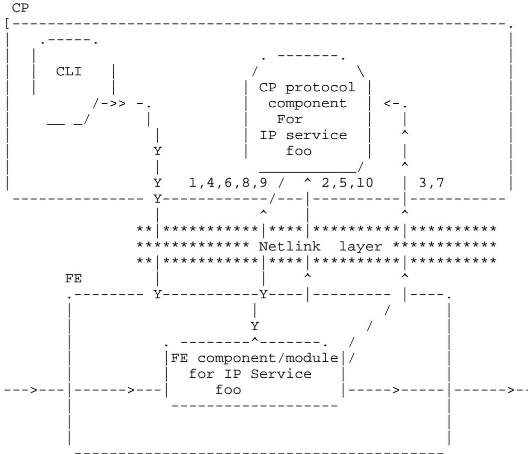
The control plane protocol for IP service foo does the following to connect to its FE counterpart. The steps below are also numbered above in the diagram.
