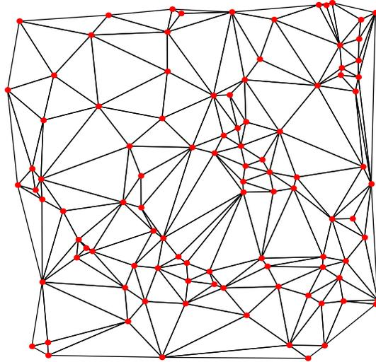
The example `Gouraudcontour.asy` illustrates how to produce color density images over such irregular triangular meshes. `Asymptote` uses a robust version of Paul Bourke’s Delaunay triangulation algorithm based on the public-domain exact arithmetic predicates written by Jonathan Shewchuk.
